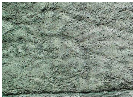
Dry Filter with Paint Contaminant
